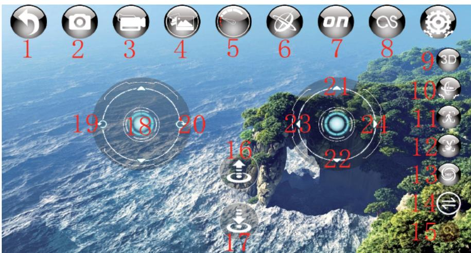
Enable G-sensor control on the control interface (icon 6 in the control interface description on above picture). When this mode is enabled, the right joystick automatically switches to control by tilting the smartphone. The controls of the left joystick remains active for the management of the altitude and rotation.
