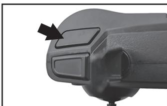
During flying, if you press headless mode button, the remote control will emit three «beep» sound, the drone's light will blink fast. The headless mode is enabled. If you press this button once again, the remote control will emit one «beep» sound, the headless mode is now disabled.
