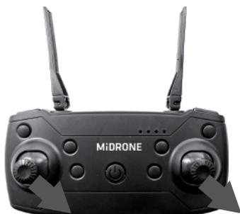
Please perform this calibration if the drone is flying unstably. This function is making a reset of the drone's gyro and of the fine adjustments (TRIM). Before calibration, it is required to place the drone on a flat surface. (If the landing gear is out of shape, the reset function will be affected). Push both joysticks as shown on the left picture, after 2 seconds the drone's lights will blink fast several times, the calibration is now completed.
