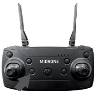
If in case of any emergency, an urgent shutdown is possible by pressing deeply (more than 2 seconds) the «Auto landing» button. (see image on the left) Do not use this function when the drone is flying normally on a high level, or the aircraft would drop down directly and get damaged.
