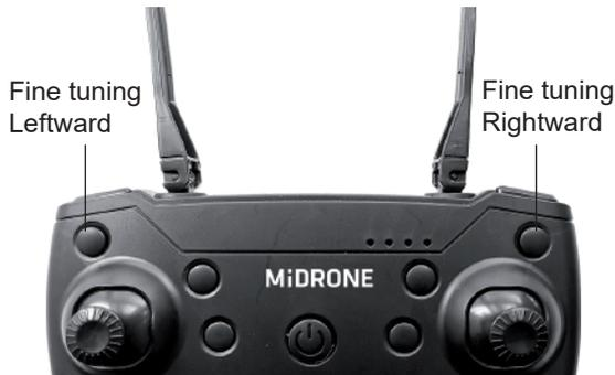
If the drone drifts rightwards in hovering flight, press the "Fine tuning leftward" button to correct it, until the drone no longer drifts.
