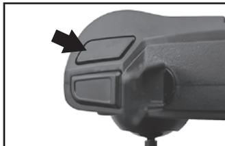
When you apply a long press to this button, the drone will fly back to the controller's position, and this function will stop when you use the right joystick to control the direction of the drone.
