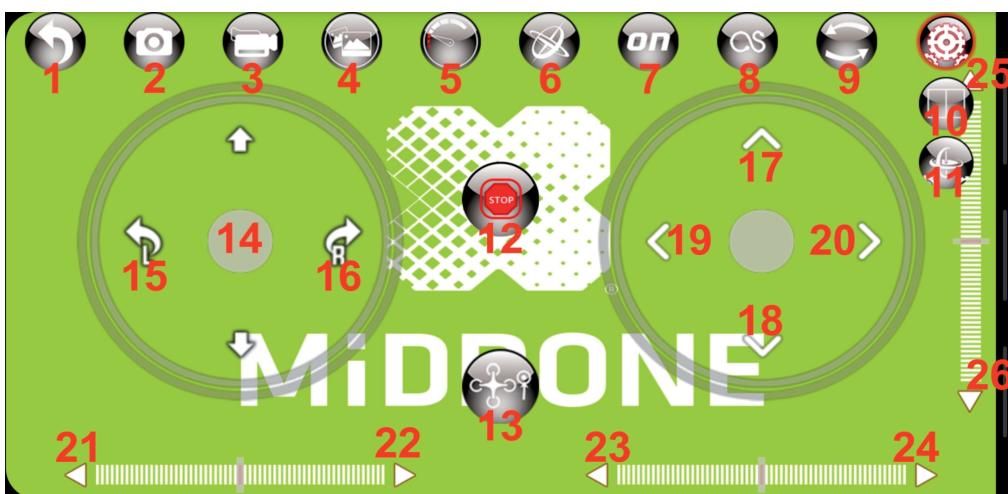
Enable G-sensor control on the control interface (icon 6 in the control interface description on above picture). When this mode is enabled, the right joystick automatically switches to control by tilting the smartphone. The controls of the left joystick remains active for the management of the altitude and rotation.
