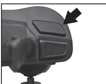
If case of any emergency, an urgent shutdown is possible by pressing deeply (more than 2 seconds) the 3D Flip button. (see image on the left) Do not use this function when the drone is flying normally on a high level, or the aircraft would drop down directly and get damaged.
