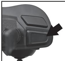
High/Low speed mode is controlling the speed of flying forward/backward/leftward/rightward. The default setting is slow mode. Press the «speed» button, the remote will emit two «beep» sound, the high speed mode is selected. Press again, this button, the remote control will emit one «beep» sound and the drone will back to slow speed mode.
