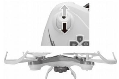
Before each flight you must establish the link between the drone and remote control by performing this operation: Push the left joystick fully upward and then pull it to the bottom. A beep sounds when the joystick is at the top and another beep when it is at the bottom. The 2 beeps indicate that the synchronization is successful and that the drone is ready to fly.
