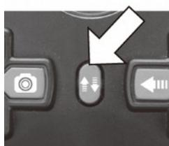
2. Once this step is done and the drone is flying, press the mode switch button on the remote control to activate CF Mode / Direction Lock. The remote will beep (2 beeps) and the LED lights of the drone will flash quickly to confirm that this mode is engaged.
