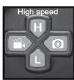
Please make sure that a micro SD card is inserted in the camera slot before taking photos and videos. The card must be SDHC type of max. 32GB and must be formatted in FAT32 file format. Press Photo button once to take a picture. Press video button once to start recording video. Press this button again to stop recording.
