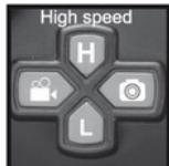
The H and L buttons are used to change the flight speed forwards / backwards / leftwards / rightwards of the drone. The default setting when the remote is turned off is on low speed. Press H button, the remote will beep twice to warn that the high speed mode is selected. Press L button, the remote will beep once to warn that the low speed mode is selected.
