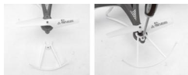
If a propeller replacement is necessary pay special attention to the direction of rotation. More details in the illustration at right. The propellers that rotate clockwise are marked with a letter A. Those that rotate in the anti-clockwise direction are marked with a letter B.
